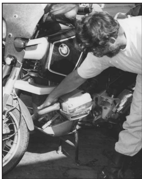
Editor Fulton Martin is pointing to the carefully engineered piece of wood that is wired so as to hold the oil level sight glass in place on the mighty 1100GS. After miles of trails in the Sawtooth Mountains of Idaho, braving forest fires and rocks, the darn glass fell out. Fellow Nez Perce riders helped with the jury-rig solution which did indeed see him safely back to San Diego.
