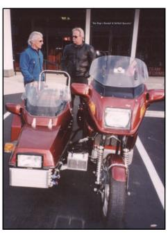
Doc Williams and John Sullivan are commenting on Jim Benge's sidecar rig. It does have a K engine and fairing, and EML frame, and Benge oil and gas coolers. It also has a nice looking expanded aluminum K-bike gas tank. (John is city engineer of Ontario.)
