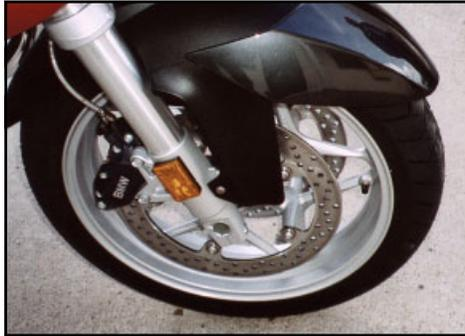
An interesting detail is the front wheel valve stem. It's in the spoke. In this picture, it's at 3 o'clock.
