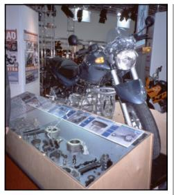
*Motorrad* had tested one for 30,000 miles and then disassembled it to find if there was any wear. The only wear they found was at the plastic timing chain tensioner.
