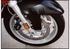
An interesting detail is the front wheel valve stem. It's in the spoke. In this picture, it's at 3 o'clock.
